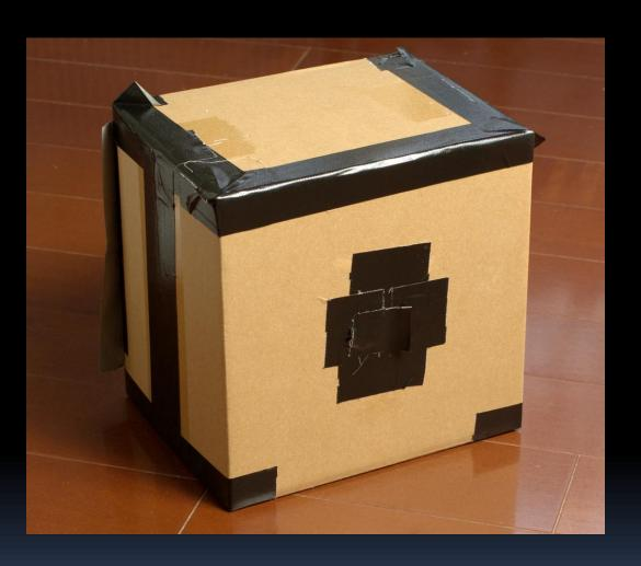
The pinhole camera is a light tight box with a small hole on one side. The media, (light sensitive material, either film or photographic paper) is placed inside. When exposed a photographic negative will result inside the box on the photographic media.
